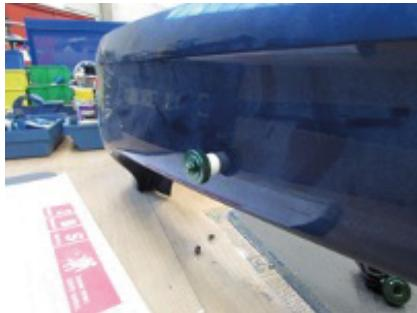
Please apply a sufficient amount of adhesive substance to the intended point on the bracket. Then position the bracket as shown on the photograph. Permanent fixing is achieved with the black clamp fitting and a knurled nut.
