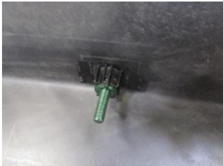
After curing, please dismantle the holding fixture and remove any glue remnants from it.
