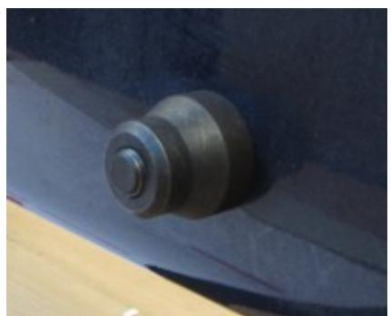
Turn the screw with an appropriate tool and make sure that the counter-piece of the hole punch does not turn on the outside.
